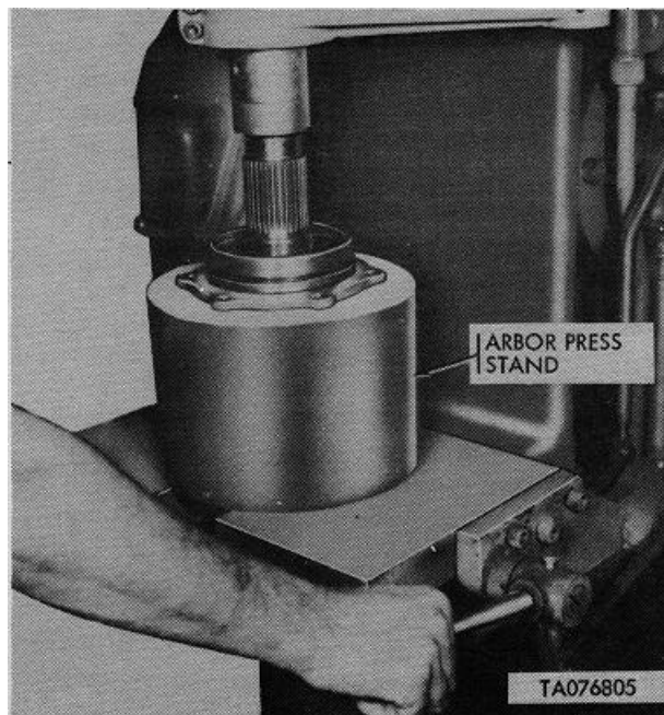
Figure 4-28. Output Shaft Removal from Bearing Cap Using Arbor Press Stand
